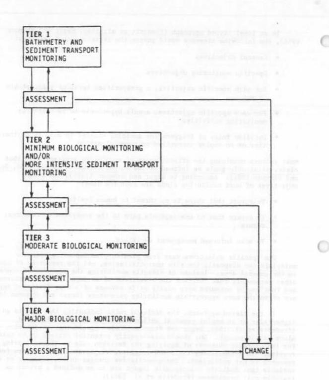
FIGURE 2. A Generalized, Tiered Approach to Monitoring Disposal of Dredged Materials
